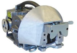
Like all the DCD lashers, the Eagle does not need traction from the strand; it uses the tension from the lashing wire to drive rotation. This lasher uses industry standard straight-hub wire spools that are loaded into a pair of drop down magazine for added convenience. The lasher will also work with standard stainless lashing or non-metallic lashing wire.
