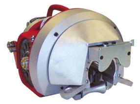
The Lineman™ Lasher holds up to 1200' per coil of 0.045" lashing wire without reloading, and works compatibly with up to 1/2" strands. A flat base ensures the lasher won't roll around in transit, and the ergonomic handle and controls add to total precision performance.
