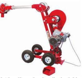
Note: This product is not to be used for any purpose other than pulling cable through conduit. A duct guide must always be used in order to lock the unit into position – without this, it is possible or likely that the entire unit will lift off the floor and may cause damage or severe injury.
