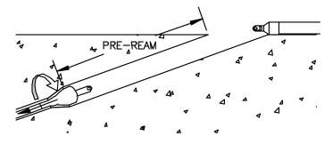
**Step 1** Pre-ream hole to minimum of one drill rod length.
