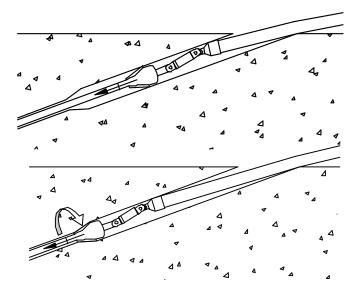
**Step 3** Pull back <u>without rotation</u> for the length of the pre-reamed hole.
